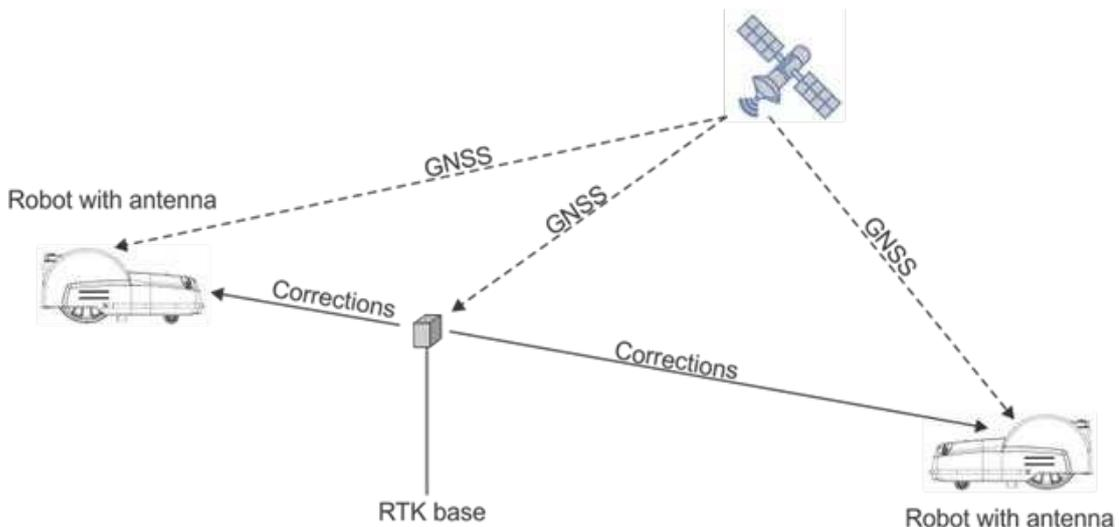
**Figure 24: Transfer of corrections using WiFi**
