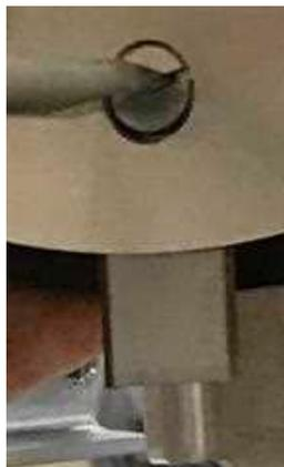
2. Undo the screw to remove the blade.
