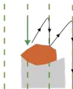
**Figure 17: Manoeuvres to avoid a large obstacle in pattern mowing**
