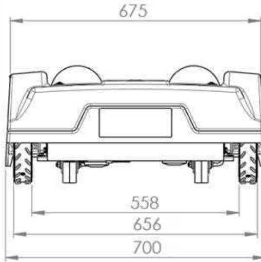
**Figure 28: Robot rear width dimensions**
