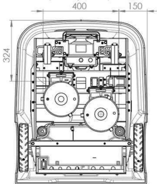
**Figure 29: Robot bottom dimensions**
