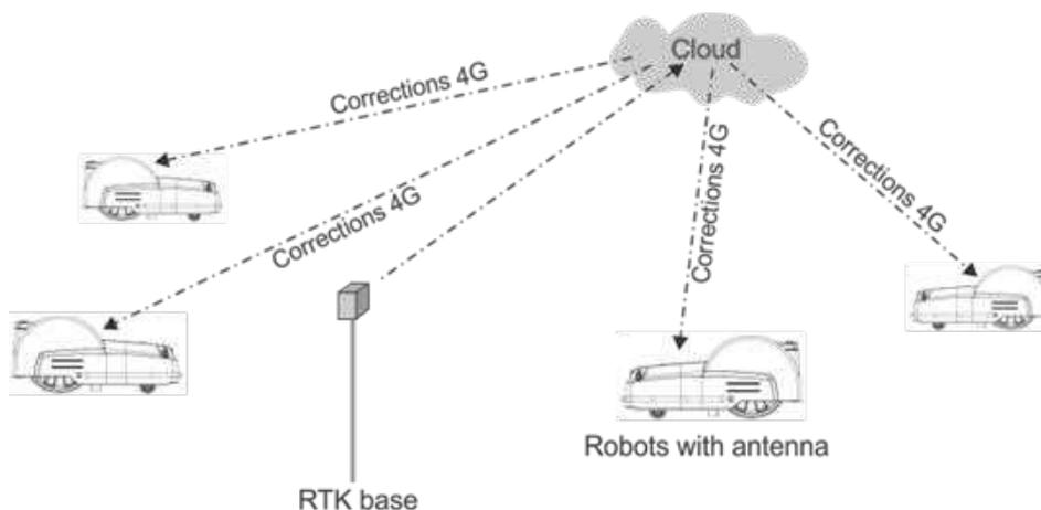
**Figure 25: Transfer of corrections using 4G**
