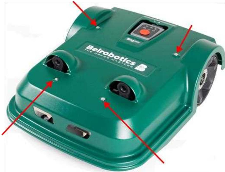
Figure 22: Body shell attachment points
