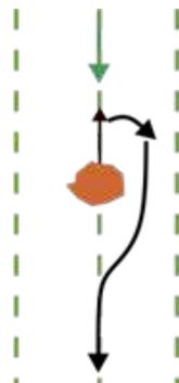
**Figure 16: Manoeuvres to avoid a small obstacle in pattern mowing**
