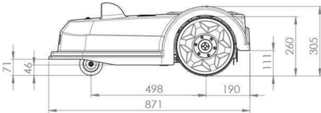
**Figure 26: Robot length dimensions**
