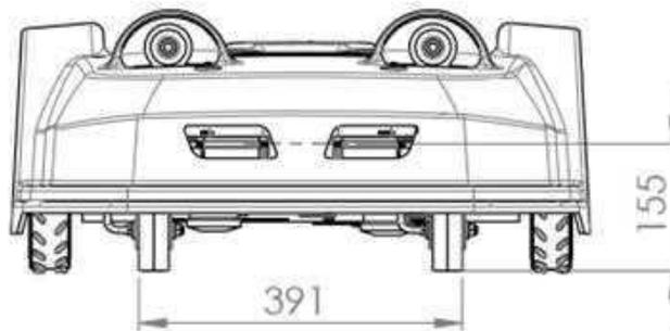
**Figure 27: Robot front width dimensions**
